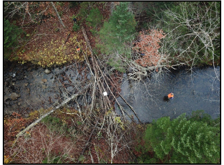
Aerial view of a strategic wood addition structure two years after installation on Tim Carroll Brook in northeastern Vermont, Photo Credit: Jud Kratzer, VFWD
